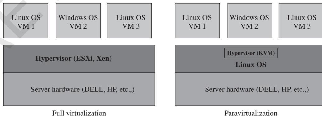
FIGURE 9.1 Two resource virtualization methods. Source: Ronglui Cao.
