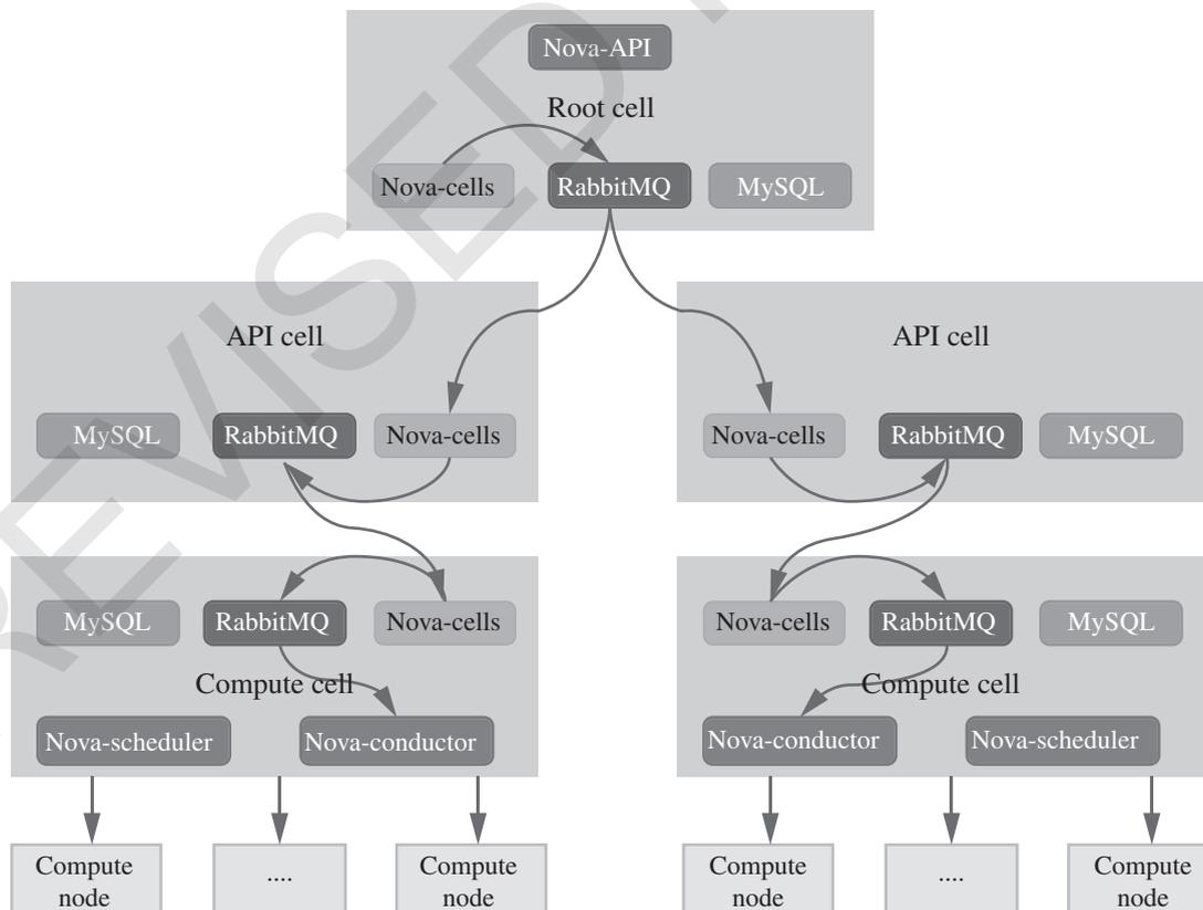
FIGURE 9.5 Nova cell architecture. Source: Rongluei Cao.
