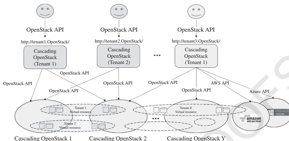
FIGURE 9.6 OpenStack cascading architecture. Source: Rongluei Cao.
