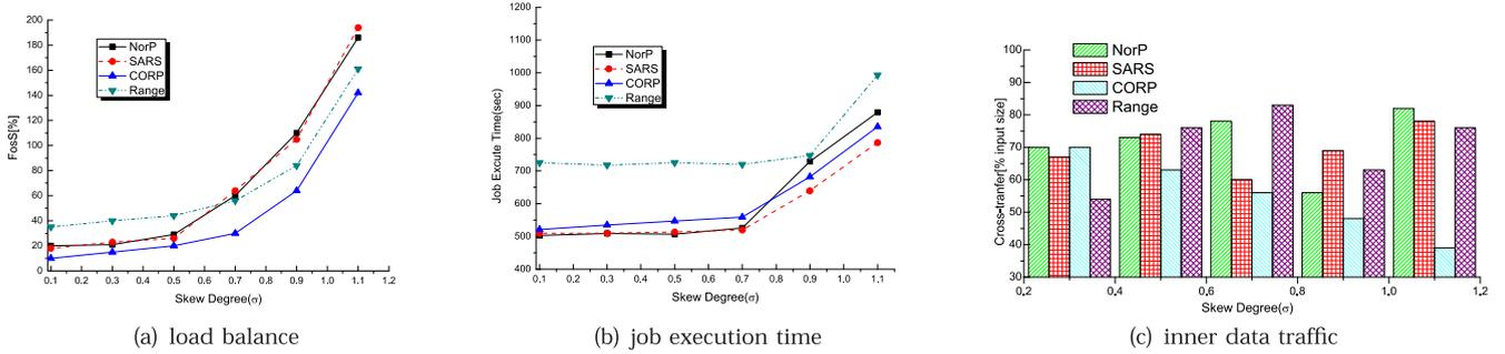
Fig. 6. Performance versus data skew for *Sort*.
