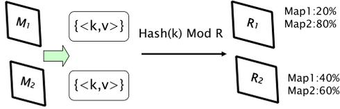
Fig. 3. The intermediate results distribution in reduce tasks.
