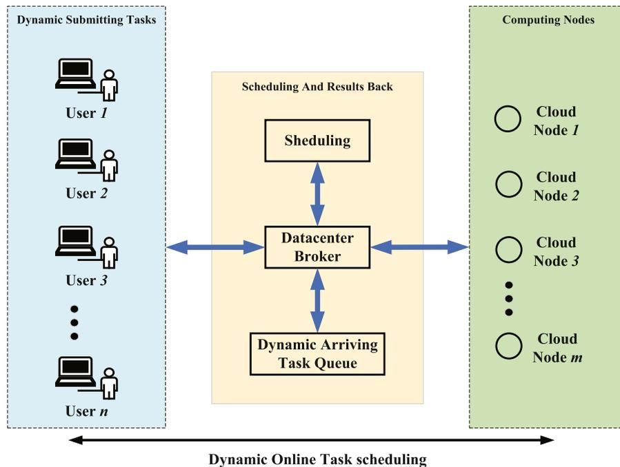
Fig. 1. Model of task scheduling in cloud computing.
