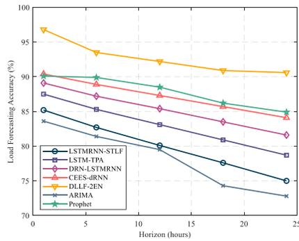
Fig. 5. Load forecasting accuracy for different prediction horizons.
