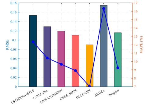
Fig. 4. RMSE and MAPE for load forecasting comparison.
