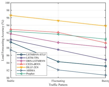
Fig. 6. Load forecasting accuracy under different network traffic patterns.
