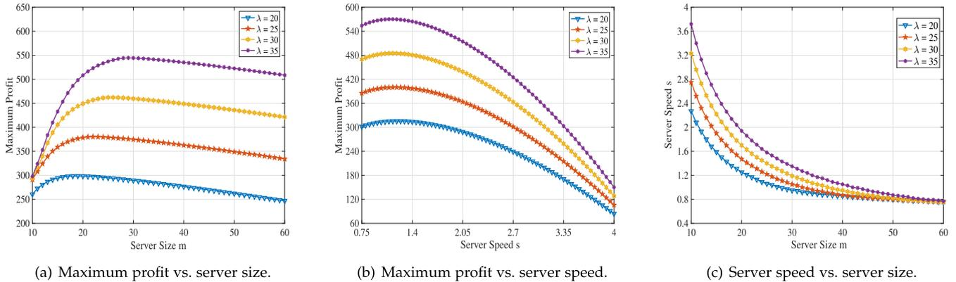
Fig. 4. Maximum profit and optimal multiserver configuration under varying service request arrival rates.
