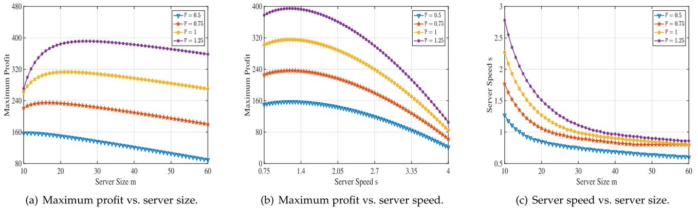
Fig. 5. Maximum profit and optimal multiserver configuration under varying expected numbers of instructions for requests.
