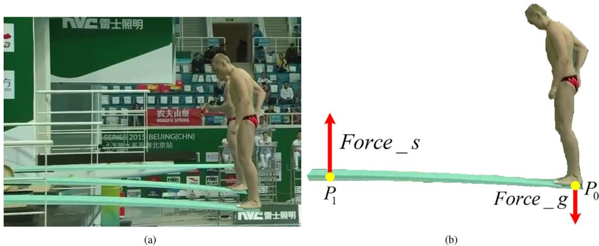
**Fig. 7.** Mechanical analysis for diving board. (a) The image with athlete standing on the diving board, (b) mechanical analysis for the diving board.
