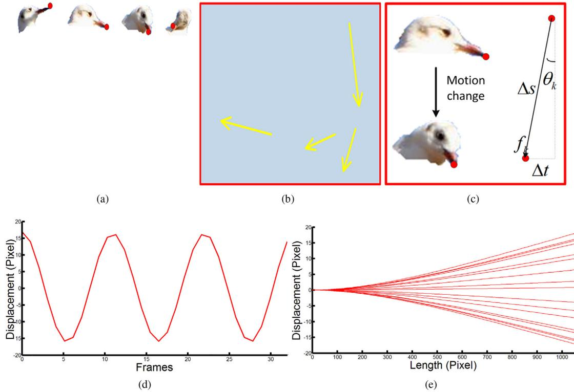
**Fig. 6.** Mechanical analysis process for seagull head shaking. (a) an example for seagull head shaking list, where the red points are the reference points of movement of the heads; (b) the velocity field of head motion of (a); (c) an example of mechanical analysis process for the motion changing; (d) the tip displacement of tree trunk within a time period; (f) the displacement of tree trunk within a time period.
