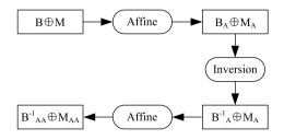
Fig. 3. The processes of mask S-box.
