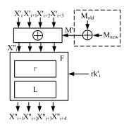
Fig. 6. The round function with update mask logic.
