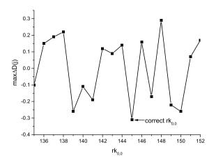
Fig. 9. DPA attack on the ordinary SM4 algorithm.
