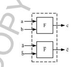
Fig. 8. The structure diagram of complementary logic.
