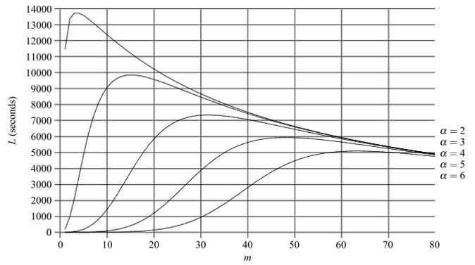
Fig. 10. Network lifetime  $L$  vs. number of annuli  $m$  (nonuniform distribution, varying  $\alpha$ ).
