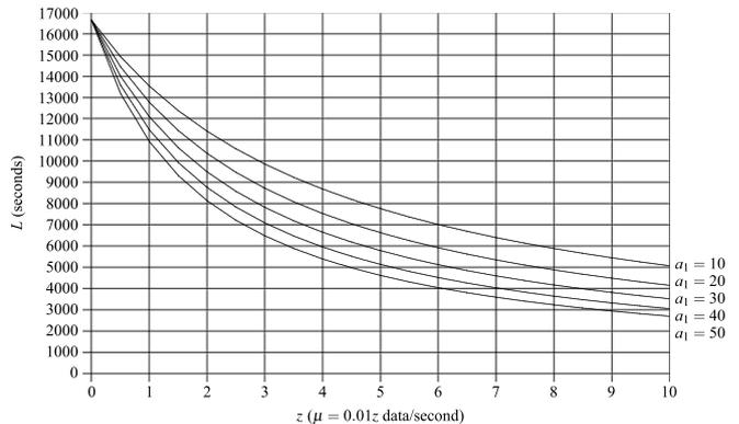
Fig. 12. Network lifetime  $L$  vs. sensor reporting rate  $\mu$  (nonuniform distribution, varying  $a$  and  $c$ ).
