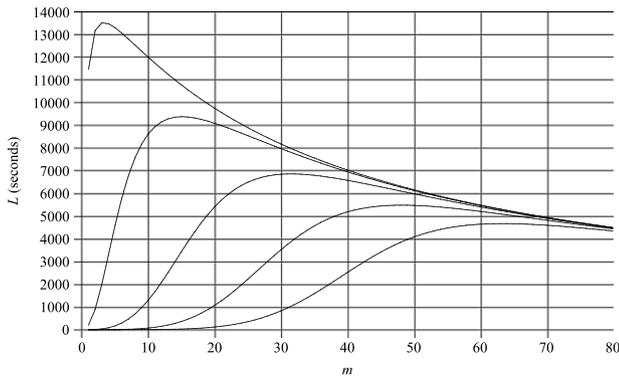
Fig. 4. Network lifetime  $L$  vs. number of annuli  $m$  (uniform distribution, varying  $\alpha$ ).
