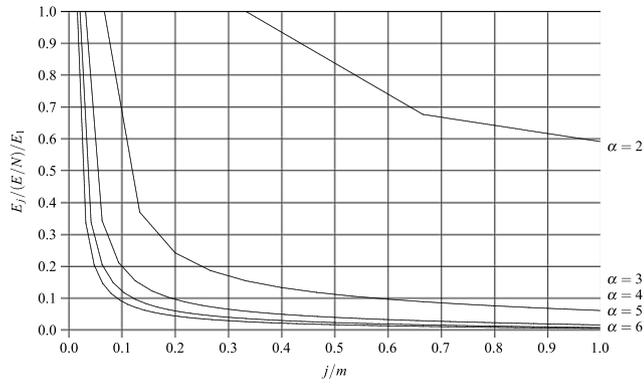
Fig. 7. Optimal energy allocation  $E_j$  vs.  $j$  (uniform distribution).
