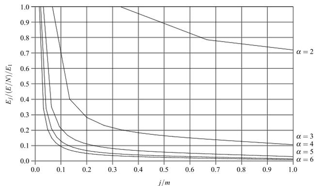
Fig. 13. Optimal energy allocation  $E_j$  vs.  $j$  (nonuniform distribution).
