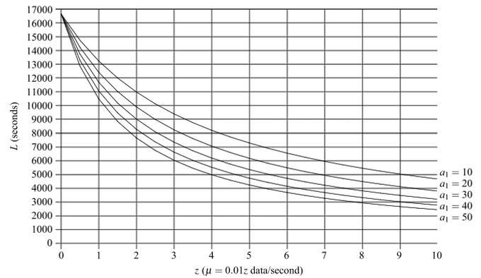
Fig. 6. Network lifetime  $L$  vs. sensor reporting rate  $\mu$  (uniform distribution, varying  $a$  and  $c$ ).
