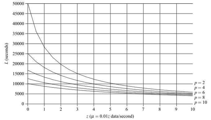
Fig. 5. Network lifetime  $L$  vs. sensor reporting rate  $\mu$  (uniform distribution, varying  $p$ ).
