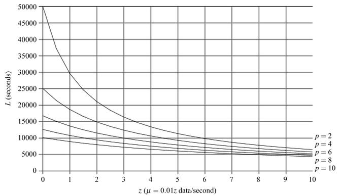
Fig. 11. Network lifetime  $L$  vs. sensor reporting rate  $\mu$  (nonuniform distribution, varying  $p$ ).
