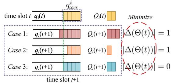
Fig. 2. Transformation process of virtual queue  $Q$ .
