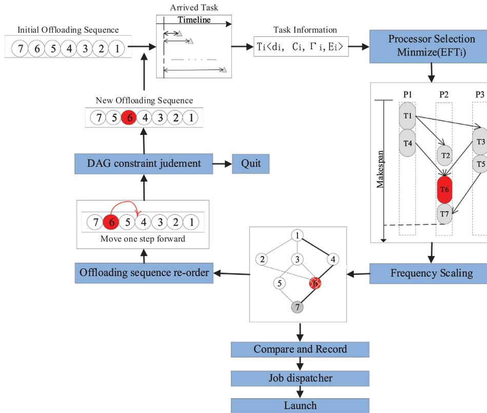
Fig. 3. Scheduler together with frequency scaling and offloading sequence re-order.
