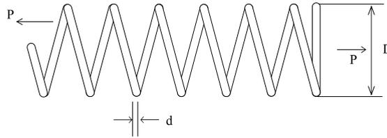
Fig. 11. Schematic view of T/CSD problem.
