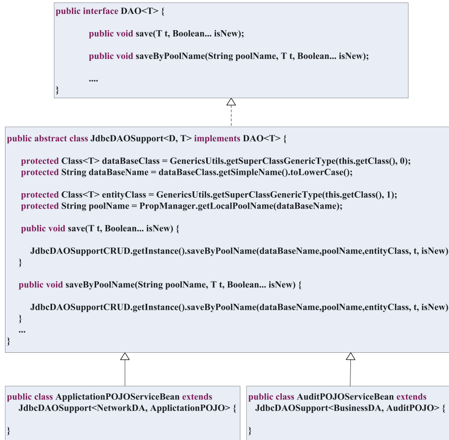
Figure 7. Data access service implemented by template method pattern. [Colour figure can be viewed at wileyonlinelibrary.com ]
