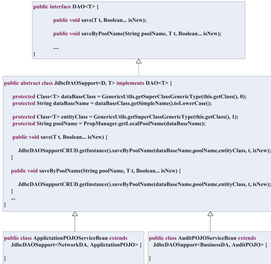
Figure 7. Data access service implemented by template method pattern. [Color figure can be viewed at wileyonlinelibrary.com ]
