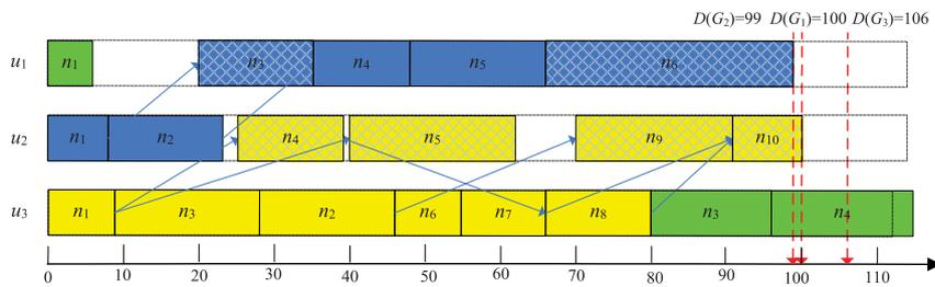
**Fig. 8.** Reusable DEWTS-generated scheduling of  $G_1$  (yellow colors) and  $G_2$  (blue colors), and  $G_3$  (green colors). (For interpretation of the references to color in this figure legend, the reader is referred to the web version of this article.)
