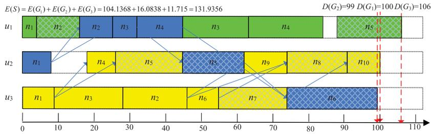
**Fig. 14.** DPMMW&GESMW-generated scheduling of  $G_1$  (yellow colors),  $G_2$  (blue colors) and  $G_3$  (green colors). (For interpretation of the references to color in this figure legend, the reader is referred to the web version of this article.)
