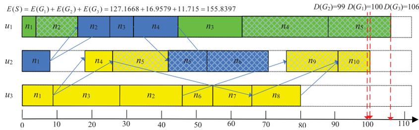
**Fig. 11.** DPMMW&EESMW-generated scheduling of  $G_1$  (yellow colors),  $G_2$  (blue colors), and  $G_3$  (green colors). (For interpretation of the references to color in this figure legend, the reader is referred to the web version of this article.)
