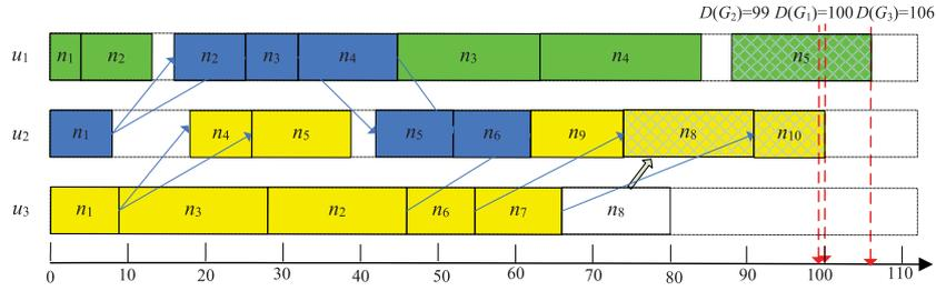
**Fig. 12.** DPMMW&GESMW-generated scheduling of  $G_1$  (yellow colors). (For interpretation of the references to color in this figure legend, the reader is referred to the web version of this article.)
