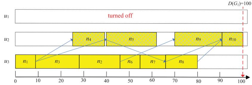
**Fig. 6.** EES-generated scheduling of  $G_1$  (yellow colors) on  $u_2$  and  $u_3$  when  $u_1$  is turned off. (For interpretation of the references to color in this figure legend, the reader is referred to the web version of this article.)
