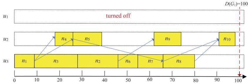
**Fig. 5.** HEFT-generated scheduling of  $G_1$  (yellow colors) on  $u_2$  and  $u_3$  when  $u_1$  is turned off. (For interpretation of the references to color in this figure legend, the reader is referred to the web version of this article.)
