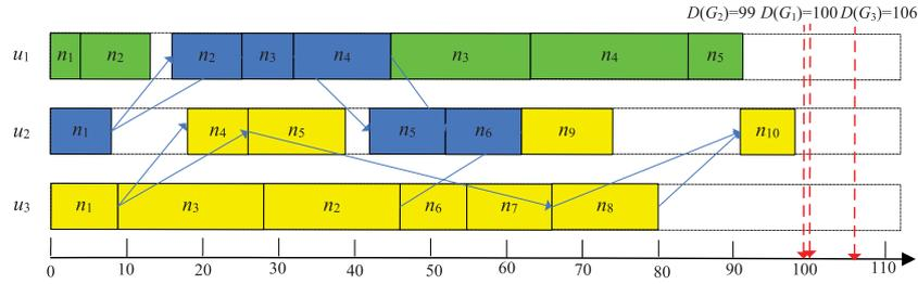
**Fig. 10.** DPMMW-generated scheduling of  $G_1$  (yellow colors),  $G_2$  (blue colors), and  $G_3$  (green colors). (For interpretation of the references to color in this figure legend, the reader is referred to the web version of this article.)
