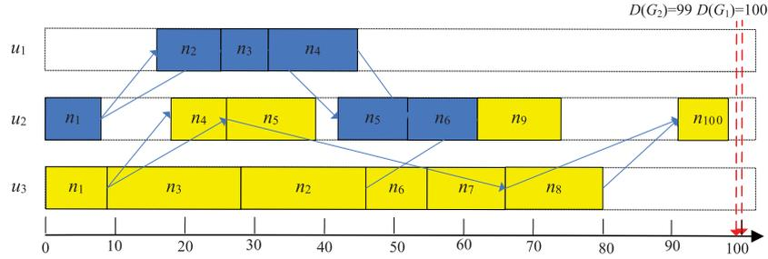
**Fig. 9.** DPMMW-generated scheduling of  $G_1$  (yellow colors) and  $G_2$  (blue colors). (For interpretation of the references to color in this figure legend, the reader is referred to the web version of this article.)
