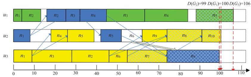
**Fig. 13.** DPMMW&GESMW-generated scheduling of  $G_1$  (yellow colors) and  $G_2$  (blue colors). (For interpretation of the references to color in this figure legend, the reader is referred to the web version of this article.)
