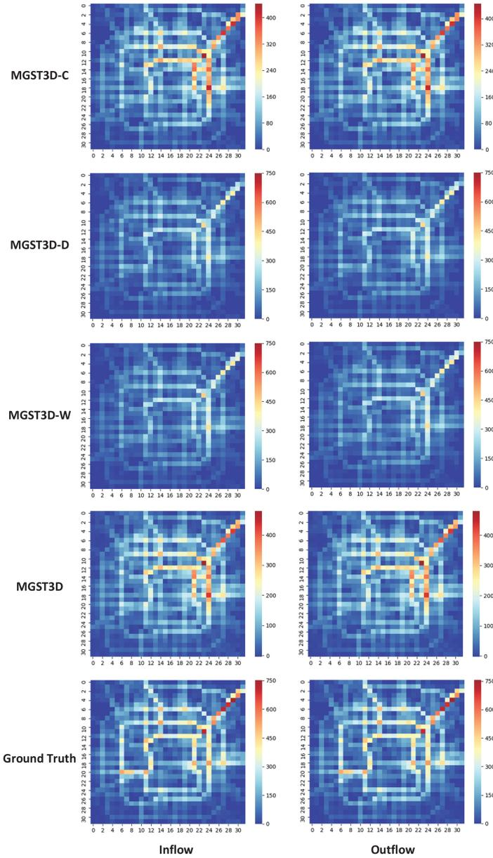
Fig. 10. Visual comparison of predicted results of different variants on TaxiBJ dataset. The top four rows are the predicted results of MGST3D-C, MGST3D-D, MGST3D-W, and MGST3D. The last row is the ground truth map. The left column is inflow maps and the right column is outflow map.
