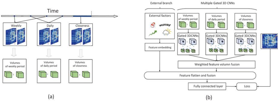
Fig. 4. (a) Modeling multiple spatio-temporal dependencies into multiple spatio-temporal 3D volumes; (b) The proposed architecture of MGSTC.
