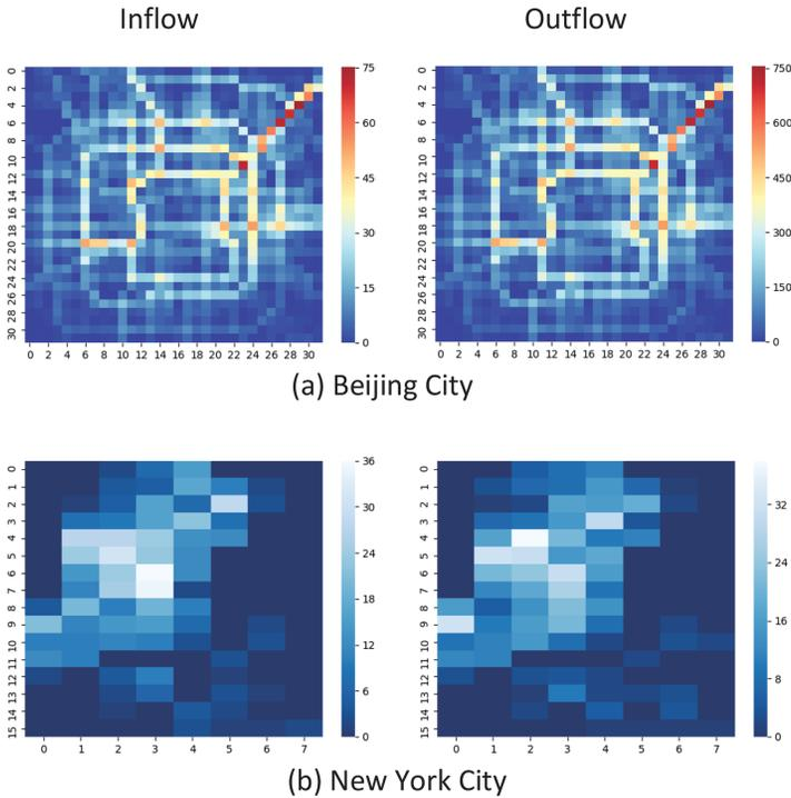
Fig. 1. Visualization of traffic flow maps in Beijing and New York City. A city is partitioned into a grid map. Two values in each grid denote the traffic inflow and outflow, respectively.
