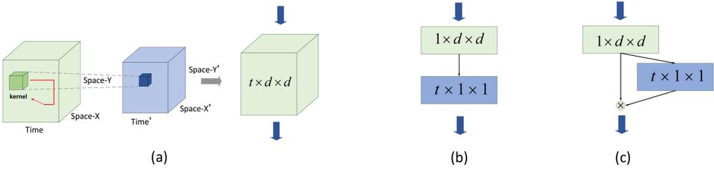
Fig. 8. Our proposed spatio-temporal convolutional blocks. (a) Extract spatio-temporal features by the original 3D CNN. (b) Our proposed spatio-temporal convolutional block without residual fusion. (c) Our proposed spatio-temporal convolutional block with residual fusion.
