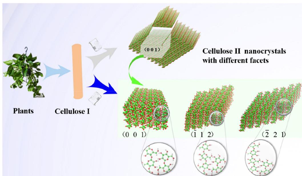
**Figure 1.** Cellulose II nanocrystals with different exposed facets. Cellulose I represent the native material in plants, from which Cellulose II can be synthesized. The facet (0 0 1) is the primary crystal facets of cellulose II nanocrystals, ( $\bar{1}$  1 2) and ( $\bar{2}$  2 1) are the inclined facets of cellulose II.
