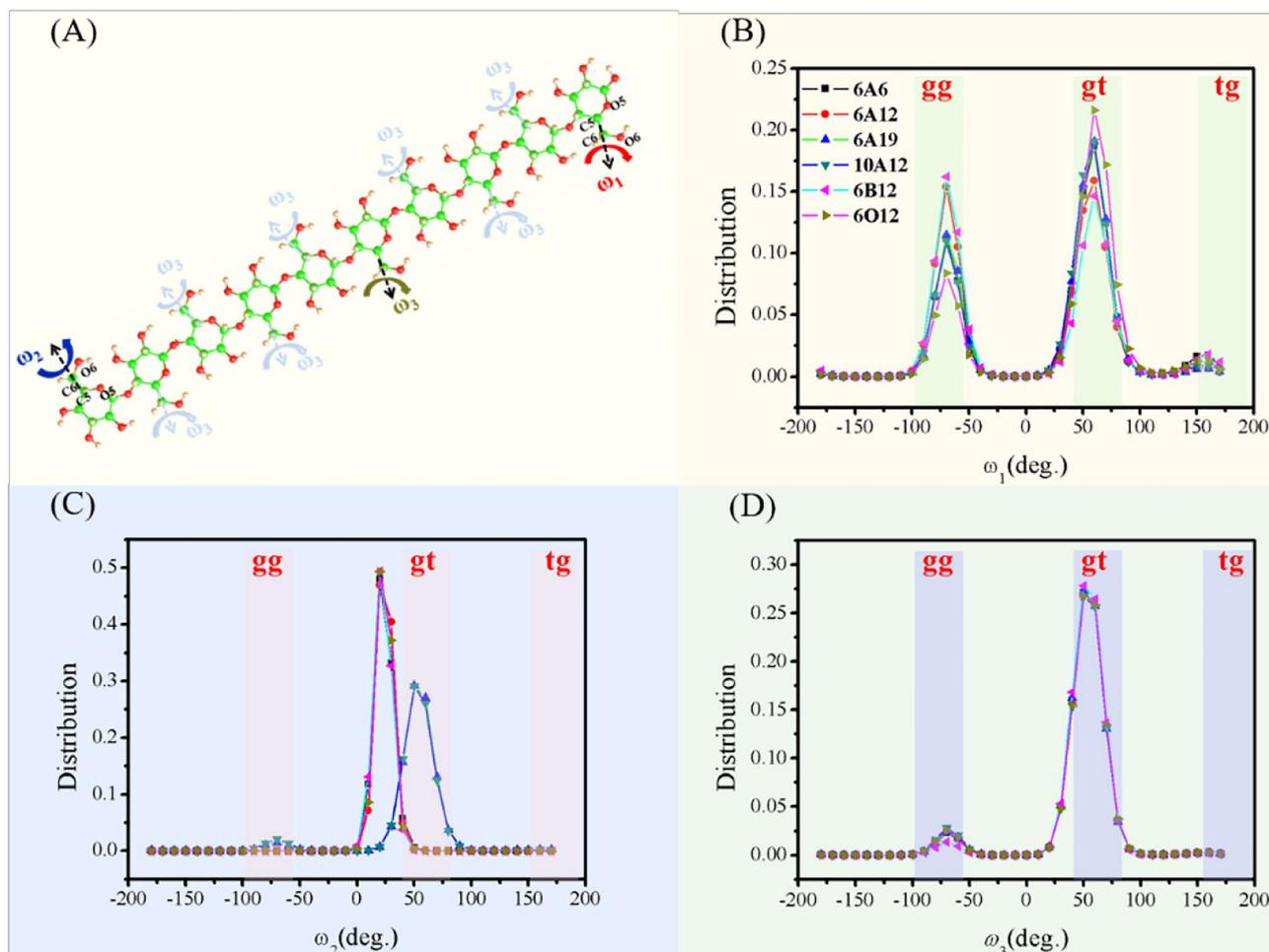
**Figure 3.** The characteristic dihedral angle  $O_5-C_5-C_6-O_6$  distribution in the MD process. (A) Definition of the torsion angle parameters of the hydroxymethyl group; (B–D) are the dihedral angles  $\omega_1$ ,  $\omega_2$  and  $\omega_3$  distributions of the residues extracted from the MD trajectories in the last 1 ns, respectively.
