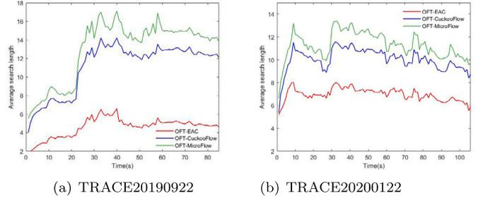
Fig. 14. The average search length of different accelerated lookup methods of virtual SDN flow table.
