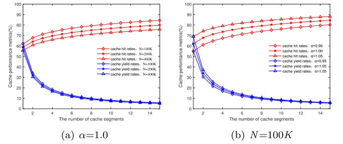
**Fig. 7.** The cache hit rate and cache yield rate with increasing number of segments.
