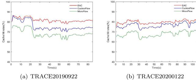
Fig. 12. The hit rates of different caches.
