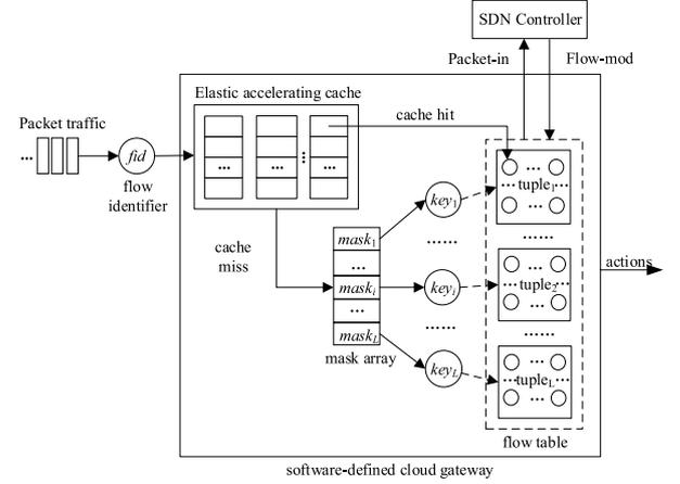
**Fig. 8.** The elastically accelerated lookup method of virtual SDN flow tables in software-defined cloud gateways.
