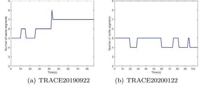
**Fig. 11.** The real-time number of segments in the EAC cache.
