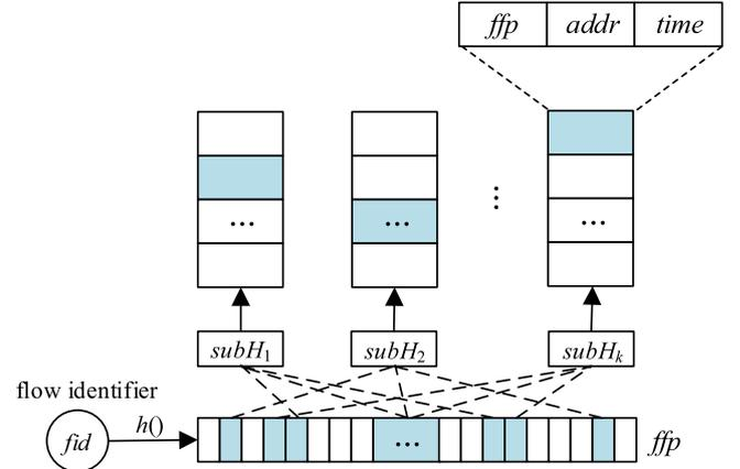
Fig. 3. Our designed elastic accelerating cache.
