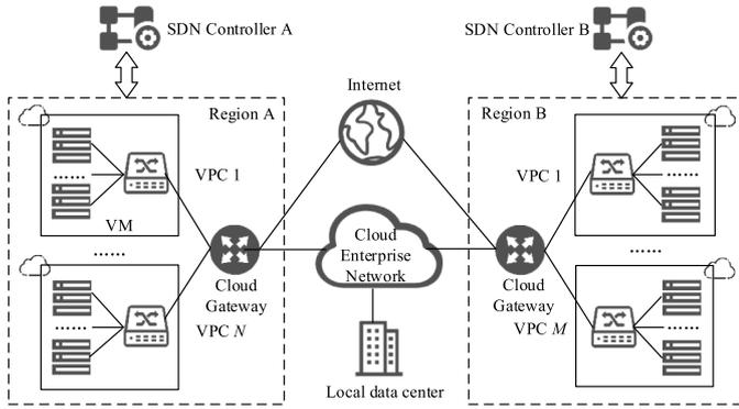
Fig. 1. A typical deployment scenario of software-defined cloud gateways.
